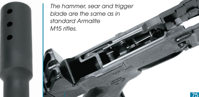
The barrel of the AR-180B features a 1:9" twist and a fixed muzzle brake with six ports.
