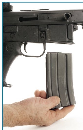
Unlike the first-generation gun, the new AR-180B takes standard AR-15 magazines.
